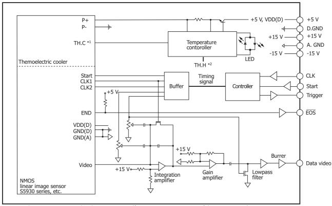
\*1: Thermistor incorporated in the image sensor (for temperature monitoring of the image sensor) \*2: Thermistor mounted on the heatsink fins (for temperature monitoring of the heat radiating side)
